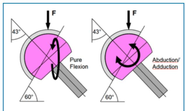
Fig. 2: Moments stress test (frictional torsion test using rotation and bending) under approximately in vivo conditions in the hip simulator<sup>8</sup> (Source: CeramTec)
