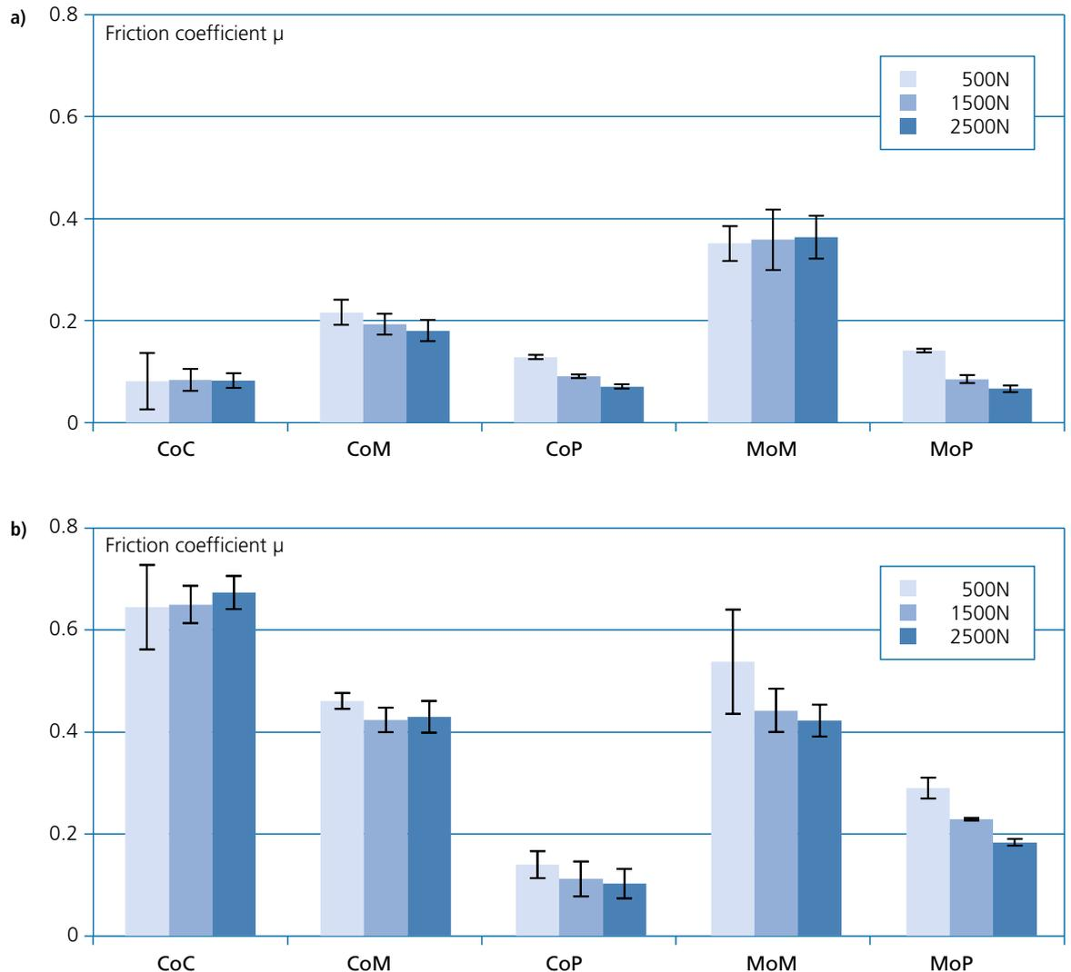
Fig. 2a, 2b: Friction coefficients for various material couples in (a) lubricated and (b) dry state
