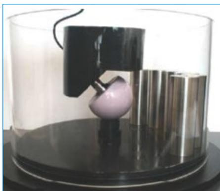
Fig. 1: Standard fretting/corrosion test in accordance with ASTM F1875 (Source: Endolab®)
