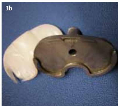
Fatigue fracture of metal condyle with corresponding polyethylene inlay wear (Fig. 3a, b)
