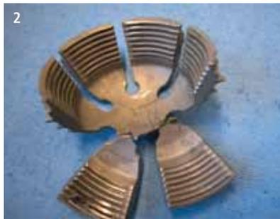
Fatigue fracture of metal stem and cup (Fig. 1, 2)
