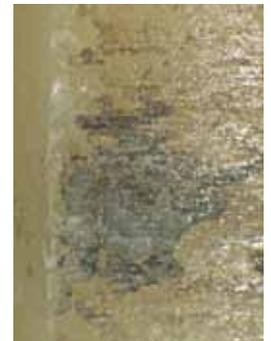
Third particles (for example, soft tissue, bits of bone and cement residue) in the taper fixation produces selective, non-planar force transmission and asymmetries in the stress-bearing area.
