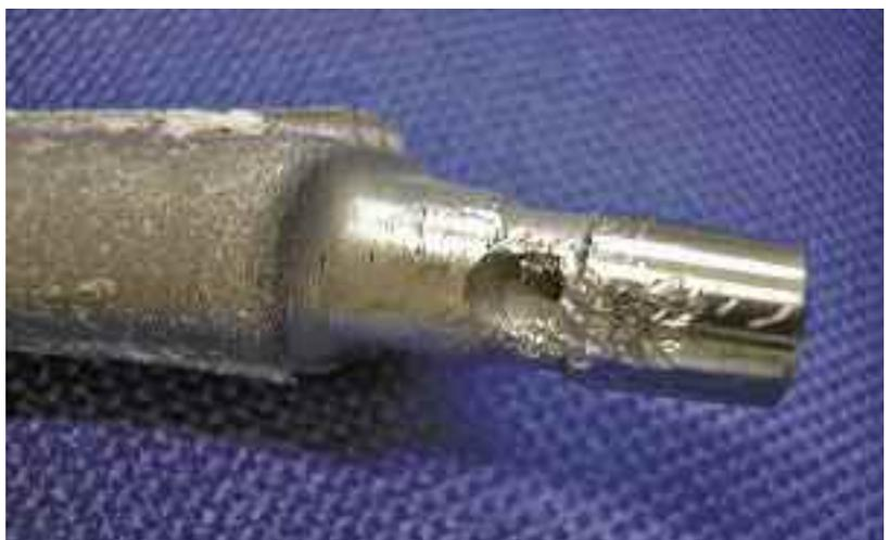
**Grade 3 taper damage: BIOLOX® OPTION cannot be used.** Photo: CeramTec AG
