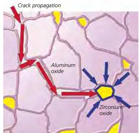
The principle of conversion reinforcement: zirconium oxide particles dissipate crack energy and absorb impacting forces.
