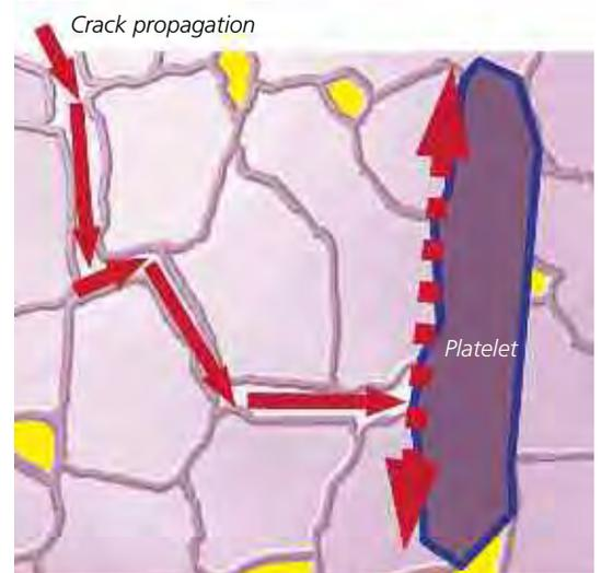
The principle of platelet reinforcement: platelet-shaped crystals block crack propagation and thereby increase the strengthening effect.
