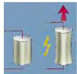
Function of piezoelectric ceramic elements
