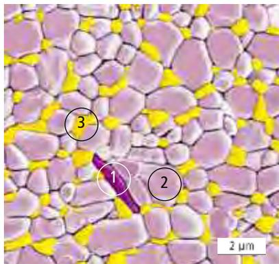
A detailed view of the BIOLOX<sup>®</sup>*delta* structure: platelets with crack-stopping function (1), aluminum oxide particle (2), zirconium oxide particle (3)
