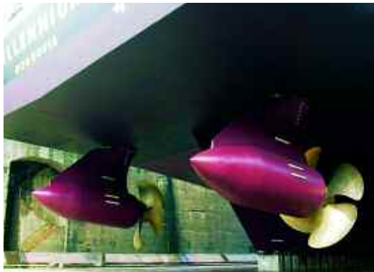
The propeller shafts on the Queen Mary 2 run on ceramic seal rings manufactured by CeramTec.
